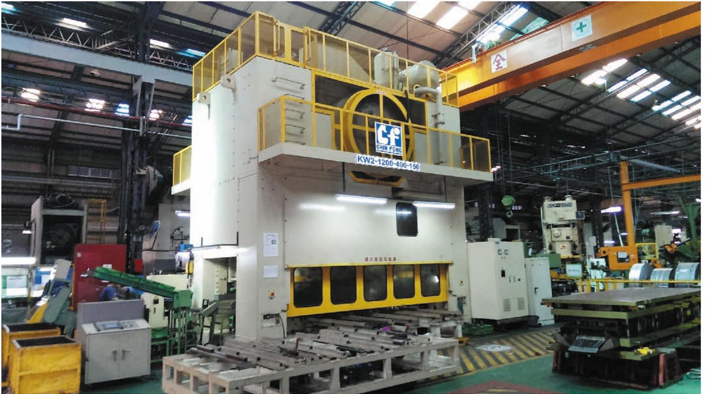
The **KW2** series press is capable of performing sheet metal stamping processes (blanking, drawing, bending, and localized forming) as well as cold forging processes (flattening/upsetting, extrusion, reduction, and embossing forming). This enables combined processes to achieve near-net-shape sheet metal and forging hybrid manufacturing.
